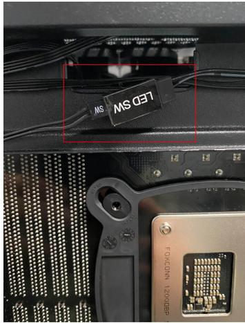
If your PC uses a any other brand of case, and the lights are not working, open the front of the case check to make sure the 5V RGB cable did not come unplugged during shipping.
