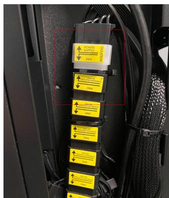
If the case lights are not changing colors when pressing the LED button, check to make sure the LED cable is properly connected.
